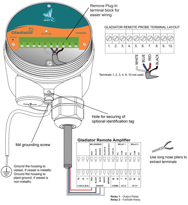
\*AC-In is replaced by 36-60VDC with Power Input Option 'C'.
