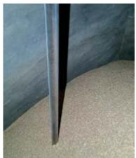
Continuous filling with build-up on probe
